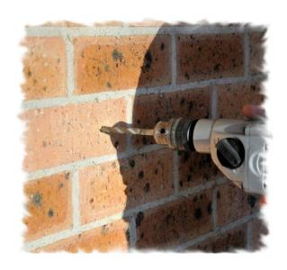
You should also use a drill that has a **hammer** or **percussion** setting, unless you're drilling into soft material such as mortar joints between bricks.
