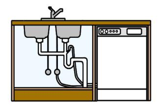
The powerpoint needs to be freely accessible without having to remove the dishwasher. This means that you'll need to cut access holes into the sink cabinet for the water hose, electrical lead and waste hose.
