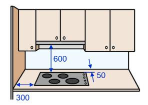
Secondly, there must be at least 50 mm clearance from the back edge of the cooktop to a non-combustible wall surface or splashback. Non-combustible surfaces include tiles, glass, stainless steel and stone.
