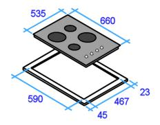
The diagram at left shows the cooktop dimensions and cut-out dimensions.
