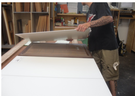
Glass being fitted to a timber framed door with a Ply insert at Team & factory Reid Austria
