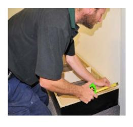
When you look closely at the end of a normal retractable tape, you'll notice that the steel hook is secured with rivets, with a bit of play in the holes allowing it to move back and forth. The amount of movement allowed is the same as the thickness of the hook.
