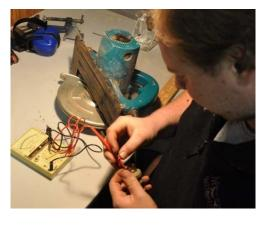
All power tools used at work need to be tested and tagged every three months by an authorised person. The test is designed to ensure that the tools are safe and not likely to cause a fire or electric shock.
