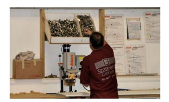
Make sure that hinges, draw runners and other components with left and right hand variations are the correct ones for the job. Check that the colour and texture are right, and that all sets are matched correctly. Also check that there are no scratches or blemishes on items that will be visible in the finished project.
