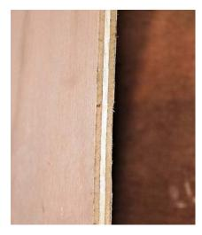
Plywood is made of thin sheets of timber veneer bonded together with formaldehyde resin. Every second veneer is laid with the grain running at right angles to the layers above and below. This is what makes plywood strong in all directions, and able to be nailed close to the edge without splitting.
