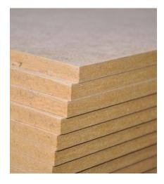
Particleboard, also called **chipboard**, is made of wood particles bonded together with a synthetic resin. It is very stable and has reasonable strength when used as panelling and shelving, as long as it is properly supported.
