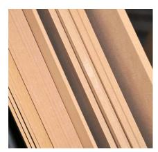
Like particleboard, MDF is also made of wood particles bonded together with formaldehyde resin. It is also available in standard and moisture resistant grades, and can be faced with different veneers.
