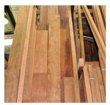
Solid timber has prestige. But it's also expensive, particularly when high grade hardwoods are used. These days, solid timber is generally limited to doors, drawer fronts, bench tops and other parts that are in full view.
