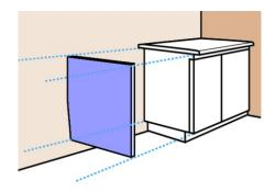
The end panel will go from the underside of the bench top to the bottom of the cabinet, above the kickboard. It will fit hard against the wall and finish flush with the front of the door. Although the wall is out of plumb, it is flat, so the tapered side of the end panel will form a straight line and won't need to be scribed.
